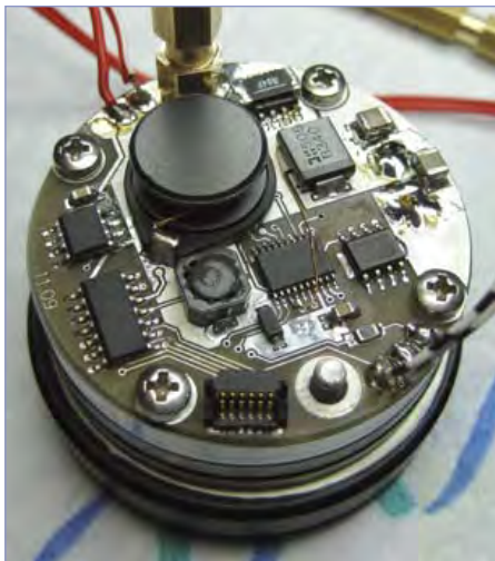
Figure 3. The circular double sided PCB takes SMD components.
