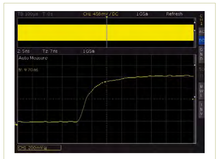
Figure 2. Fast signal changes (<10 ns) can be resolved with a one million point acquisition memory and a recording time of 1 ms.
