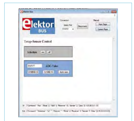
Figure 3. Display of ADC values and temperature readings in the ElektorBus browser.
